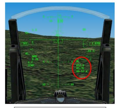
If you have the ground radar on and slew the cursors, your slant range/ETA/actual range data will be based upon the designated radar cursor location.
