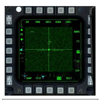
Slewing the radar cursor over the target I select the DBS1 resolution, although the cluster of buildings is too tight to discriminate individual structures.
