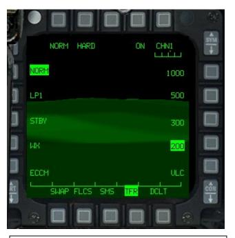
Then I pull up the TF page on the right MFD and select TFR MODE from STBY to NORM, select HARD ride mode, 200' terrain clearance, and then engage the TF (ON). My F-16 dips lower as the TF radar/autopilot takes me down for an exciting ride at 200 feet:
