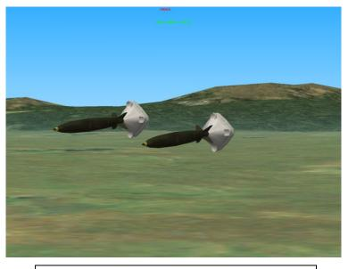
A fraction of a second later the ballutes inflate on the end of the Mk-84.
