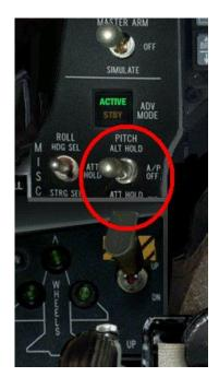
I start by turning on the auto-pilot which simply holds my barometric altitude (well above the terrain).
